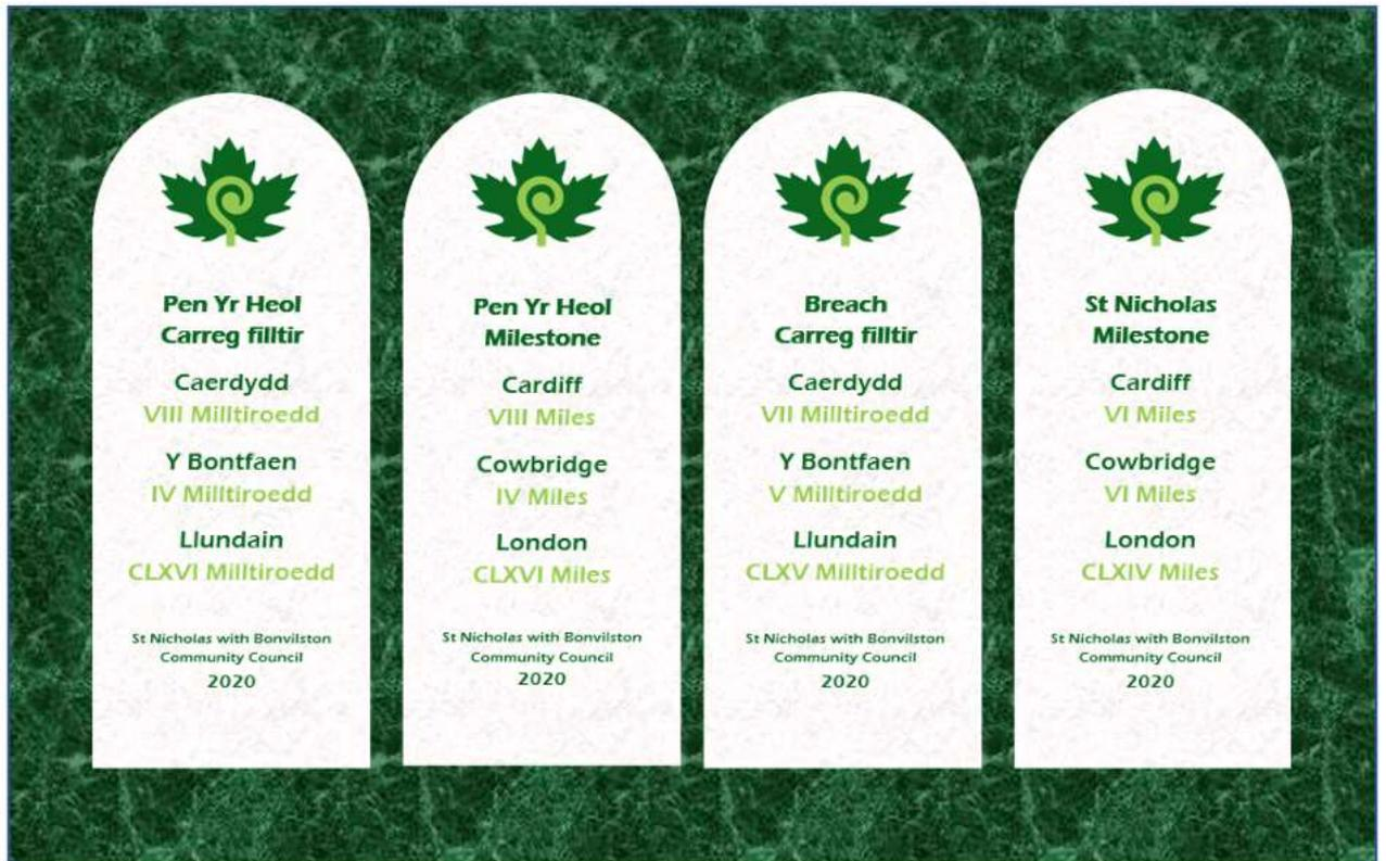
Four casts would be required, costing £400 each. The lettering and numbering imprinted into the concrete, and filled with a green resin. These would then be situated where the original milestones were placed.
